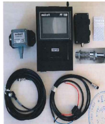
Fig. 1. Meicott Digital Monitoring sensors and units.
