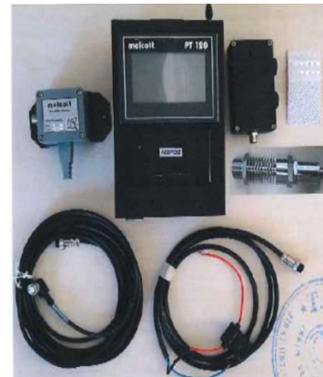
Fig. 1. Meicott Digital Monitoring sensors and units.
